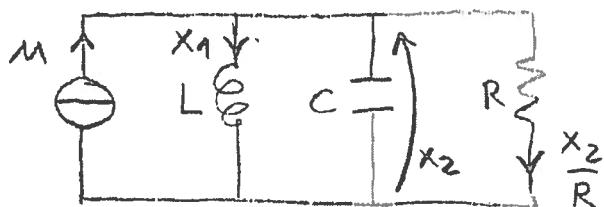
$$\left[ \begin{array}{l} i_C = C \frac{dV_C}{dt} \\ V_L = L \frac{di_L}{dt} \\ V_R = R i_R \end{array} \right] \quad \left[ \begin{array}{l} \uparrow i_C \uparrow V_C \\ T \uparrow \\ \downarrow i_L \downarrow V_L \\ R \uparrow i_R \uparrow V_R \end{array} \right]$$
