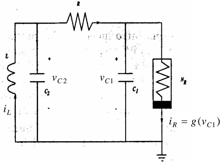
$$\begin{aligned}C_1 \frac{dv_{C1}}{dt} &= \frac{1}{R}(v_{C2} - v_{C1}) - g(v_{C1}) \\C_2 \frac{dv_{C2}}{dt} &= \frac{1}{R}(v_{C1} - v_{C2}) + i_L \\L \frac{di_L}{dt} &= -v_{C2},\end{aligned}$$
