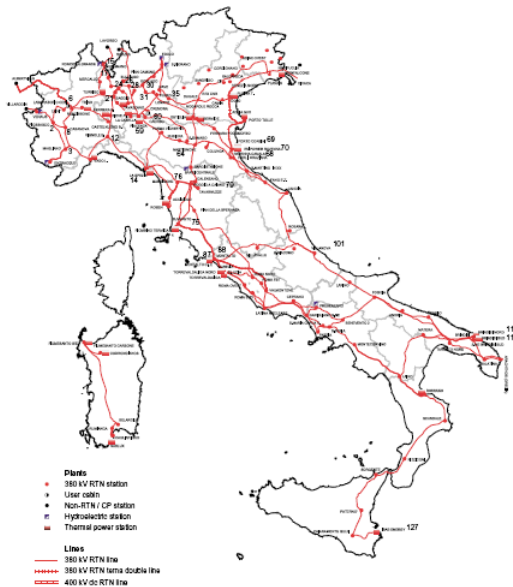
Figure 1. The 380 kV Italian power transmission network (TERNA 2002, Rosato, Bologna et al. 2007).
