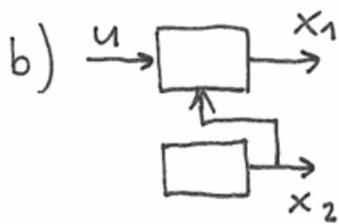
$$\begin{aligned} \dot{x}_1 &= x_1 + x_2 + u \\ \dot{x}_2 &= -x_2 \end{aligned}$$
